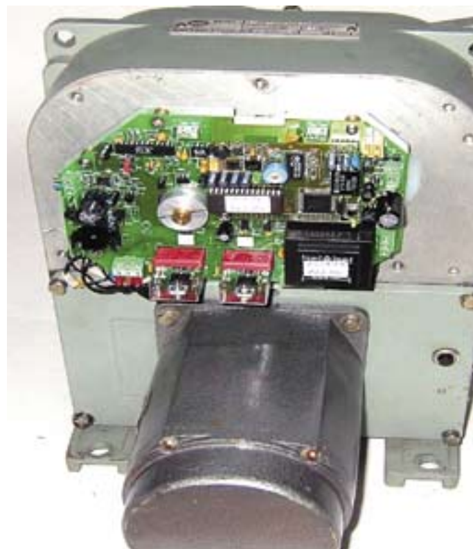
Digital (Mouvon) module with the digital positioner in the housing of the actuator.
