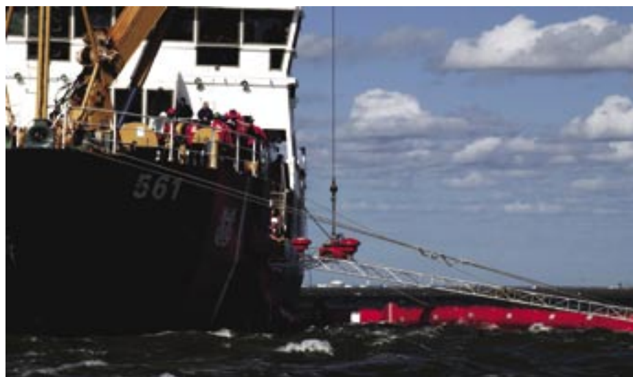
Crewmembers on board the Coast Guard Buoy Tender Harry Claiborne lower an oil skimmer into the water during a pollution response drill in Galveston Bay. The oil skimmer is a part of the Coast Guard's Vessel of Opportunity Skimming System (VOSS), along with containment boom, an inflatable oil recovery barge, and pumps and compressors to operate them. When deployed, the VOSS equipment uses containment boom to collect oil into a small area to make it easier for the skimmer to remove the oil from the surface of the water. (U.S. Coast Guard Photo)
