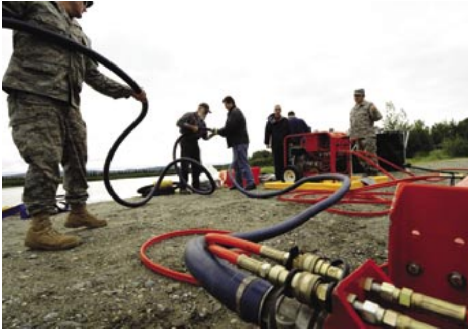
The NCOIC of liquid fuels maintenance untangles a discharge hose before connecting it to a drum skimmer in preparation for a oil and light fuels spill water contamination clean-up. (U.S Air Force Photo)
