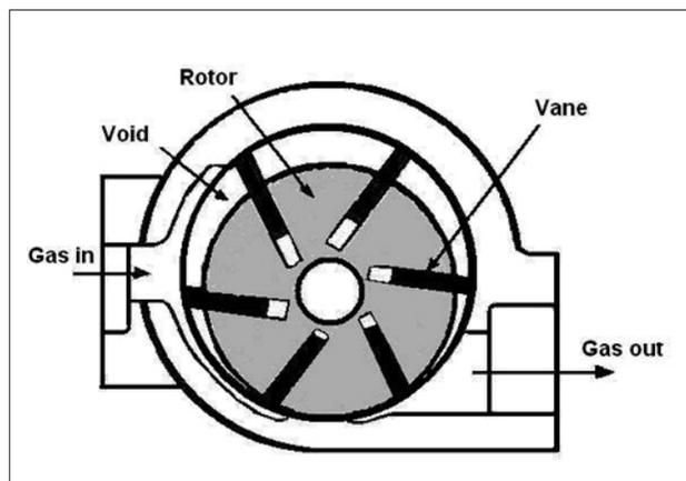
**Fig. 3: multi-cell vacuum pump.**
