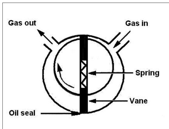
**Fig. 2: oil lubricated rotary vane vacuum pump.**
