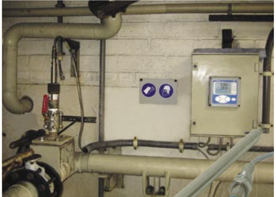
Test configuration of the pH sensor and liquid analyzer at the Hoboken plant of Umicore.
